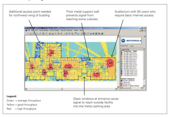
With LANPlanner, you can easily factor in the construction of your building to ensure that your wireless LAN design is optimized to deliver required performance levels in your specific environment.
